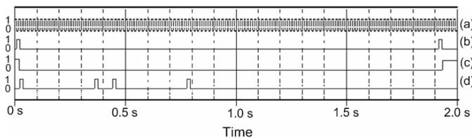
(a) Synchronous voltage square wave generated by voltage comparator
