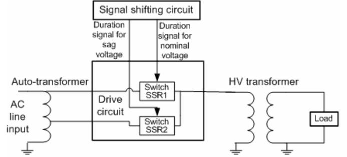
Fig. 7 The construction of the drive circuit
