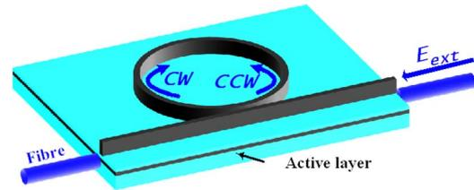
Fig. 1. Circular SRL with an external optical injection. The laser operates in the CCW direction before the optical injection ( $E_{ext}$ ) is added. It is switched to the CW direction after the injection.
