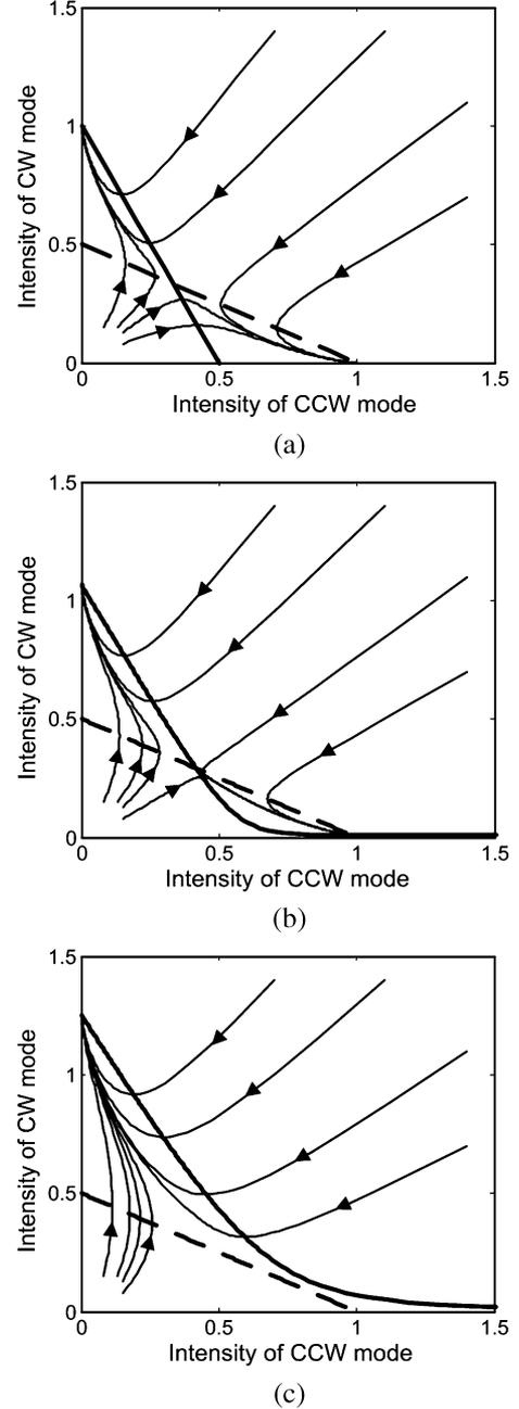
Fig. 2. Illustrations of trajectories of the intensities of CCW and CW mode (normalized to one) in the phase plane under the condition of  $\varepsilon_c = 2\varepsilon_s$ . Bold solid lines are the trajectories for  $dS_2/dS_1 = 0$ , and bold dashed lines are those for  $dS_2/dS_1 = \infty$ . (a) Without external injection. (b) With relatively low injection. (c) With adequate injection.
