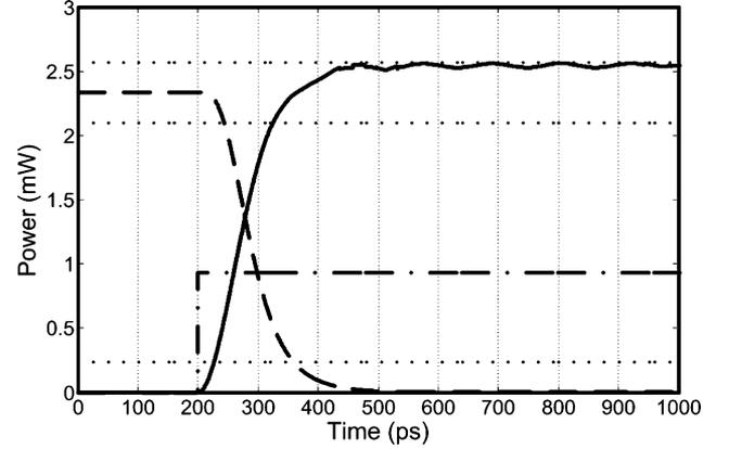
Fig. 4. Numerical transient output power of CW (solid line) and CCW (dashed line) following external optical continuous wave (dash-dotted line) injected at 200 ps, and  $\Delta\omega = -4$  GHz. The lasing direction changes from CCW (initial lasing direction) to CW (final lasing direction). The one lower and two upper dotted lines indicate the 10% margin of the initial power.
