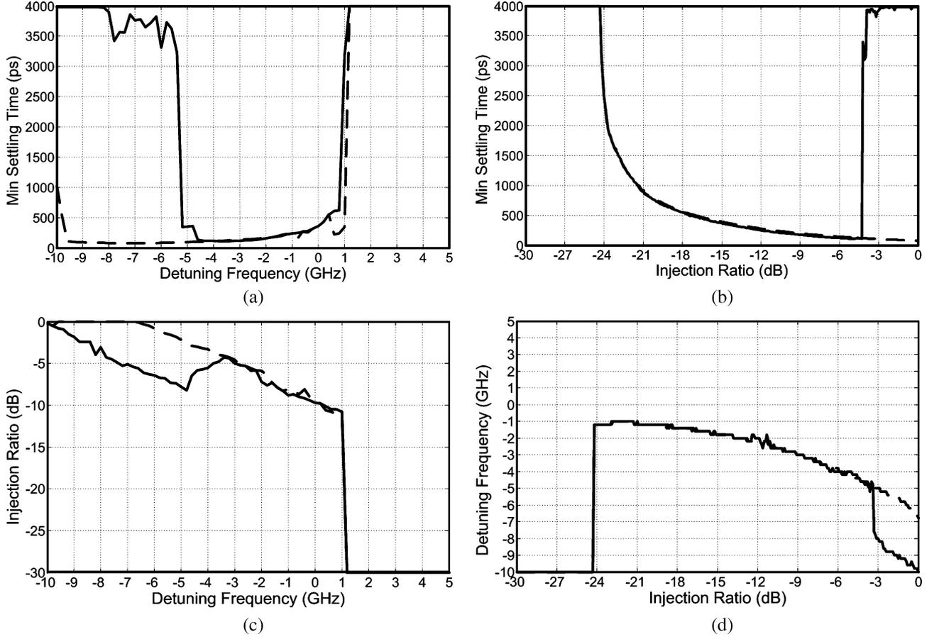
Fig. 5. Simulated minimum settling time for CW (dashed line) and CCW (solid line) (a) at different detuning frequency, (b) at different injection ratio, (c) injection ratio for minimum settling time at different detuning frequency, and (d) detuning frequency for minimum settling time at different injection ratio.
