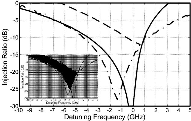
Fig. 3. Calculated minimum switched, the locking and stable locking regions. Dash-dotted line gives the minimum injection ratio required to achieve flipping for a certain detuning frequency, the locking region is outlined between two solid lines, and dashed line shows the maximum injection ratio before unstable locking. Inset figure indicates that the simulated results (middle black region) coincide with the intersection of those three regions and good agreement is achieved.
