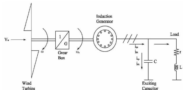
Figure (1): Wind energy conversion system
