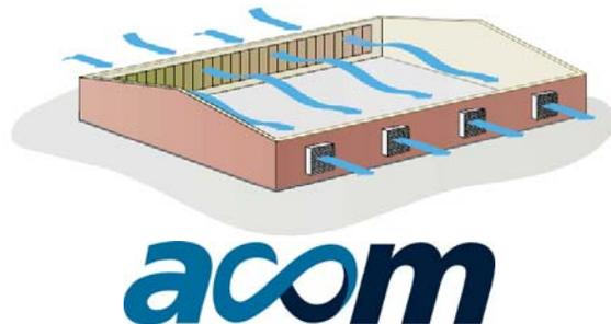
This system guarantees the uniform humidity of the refrigeration panels by the evaporation and the continuous water flow.
