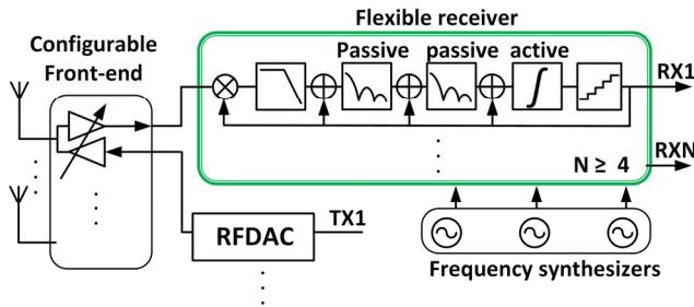
Fig. 3. The architecture of flexible transceiver.
