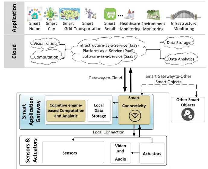
Fig. 2. Local area computing with smart application gateway.
