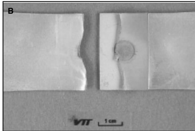
Fig. 14 — Macrographs of dissimilar metal joint EN 1.4318-ZStE260BH after SSRT test in 3.5% NaCl solution at room temperature (A) and EN 1.4318-EN 1.4318 steel sample with Zn-anode after SSRT test in 3.5% NaCl solution at room temperature (B).
