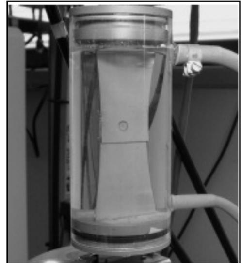
Fig. 2 — The corrosion cell used in the corrosion fatigue test.
