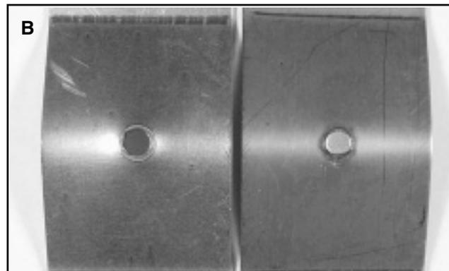
Fig. 9 — Typical plug failures. A — lap shear test; B — cross-tension test.
