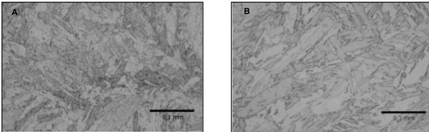
Fig. 3 — Typical martensitic microstructure of weld nugget of dissimilar metal joints. A — Stainless steel EN 1.4318 2H and nonstainless steel DX54DZ; and B — nonstainless steel DX54DZ – stainless steel EN 1.4318 2B – nonstainless steel DX54DZ.
