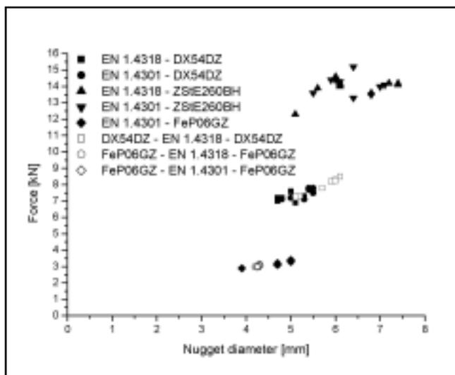
Fig. 8 — Lap shear test results of dissimilar metal joints show the effect of the different strengths and sheet thicknesses of the nonstainless steels.
