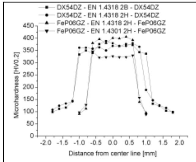
Fig. 7 — Vertical microhardness profiles of triple sheet dissimilar metal joints.
