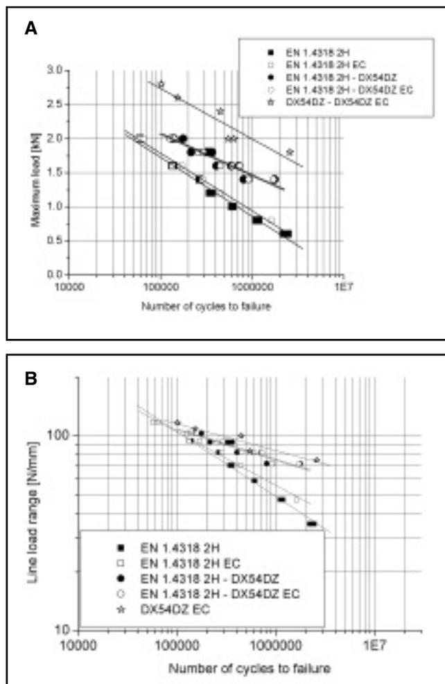
Fig. 11 — A — Corrosion fatigue test results of spot welded joints in 3.5% NaCl solution at 50°C; B — corrosion fatigue test results of spot welded joints in 3.5% NaCl solution at 50°C. Line load range analysis of the data.
