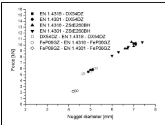
Fig. 10 — Cross-tension test results of dissimilar metal joints.
