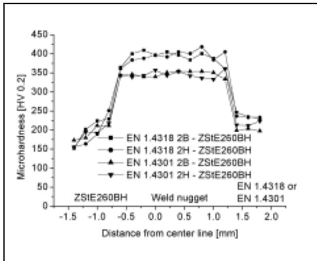
Fig. 6 — Vertical microhardness profiles of dissimilar metal joints of 1.9-mm stainless steels and 1.5-mm nonstainless steel ZStE260BH.
