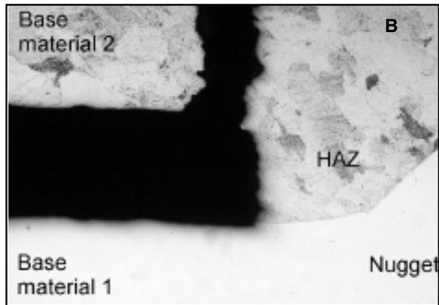
Fig. 12 — Crack initiation and growth. A — EN 1.4318 2H-EN 1.4318 2H steel joint; B — EN 1.4318 2H-DX54DZ dissimilar metal joint in the nonstainless steel side.
