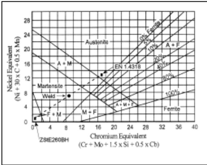
Fig. 1 — The microstructure of the weld nugget of a dissimilar metal joint EN 1.4318 – ZStE260 BH, predicted by means of the Schaeffler diagram when dilution is 50%.
