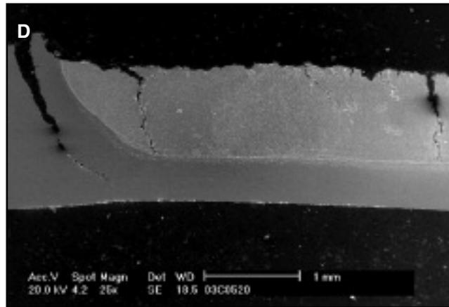
Fig. 15 — Shear loaded EN 1.4318 2B-ZStE260BH dissimilar metal joint sample after SSRT test in 23% NaCl at room temperature ( $O_2$  purging). A — Fracture in the EN 1.4318 2B side; B — fracture in the ZStE260BH side; C — fracture surface of the EN 1.4318 2B side; D — cross section of the fracture surface of the EN 1.4318 2B side.
