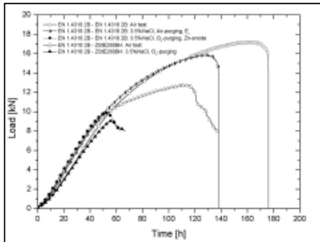
Fig. 13 — Results of the slow strain rate tests with spot welded EN 1.4318-EN 1.4318 and EN 1.4318-ZStE260BH steel joints in 3.5% NaCl solution at room temperature.
