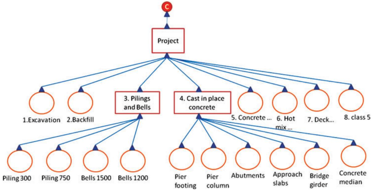
Fig. 12. Developed model for the highway overpass example using fuzzy Monte Carlo cost range estimating SPS template.
