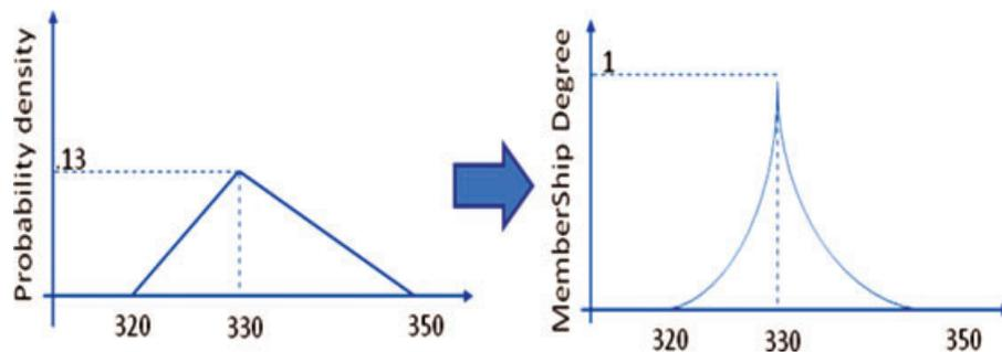
Fig. 13. Transformation of the triangular distribution for the unit cost of the pier footing process to a fuzzy membership function.
