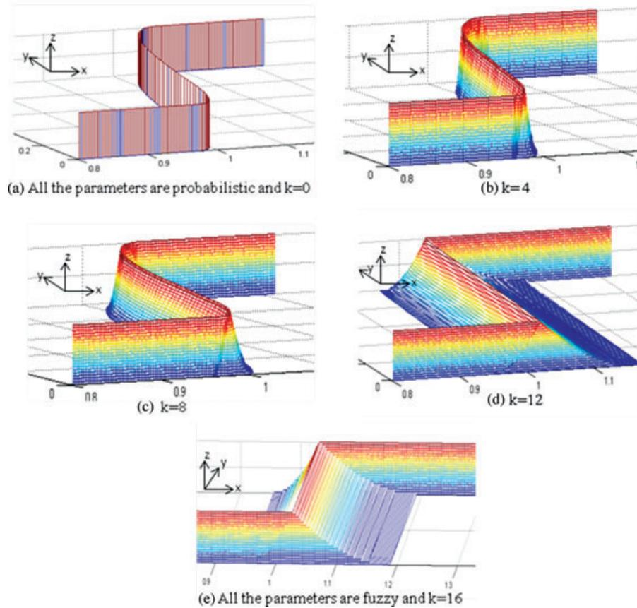
**Fig. 14.** Three-dimensional view of fuzzy CDF resulting from the output of FMCS for the highway overpass project;  $k$  indicates the number of fuzzy sets in each experiment.
