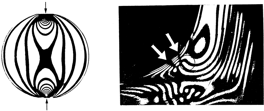
Fig. 5. Integrated fringe patterns in a light-field circular polariscope of a diametrically loaded sphere (left) and of the wall-to-bottom region of a tempered drinking glass (right, arrows indicate interference blots).
