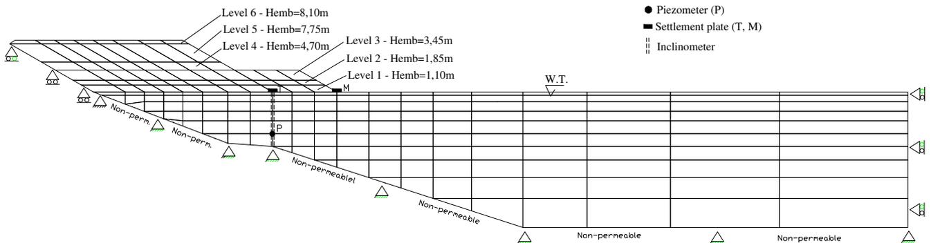
Fig. 1. Finite element mesh.
