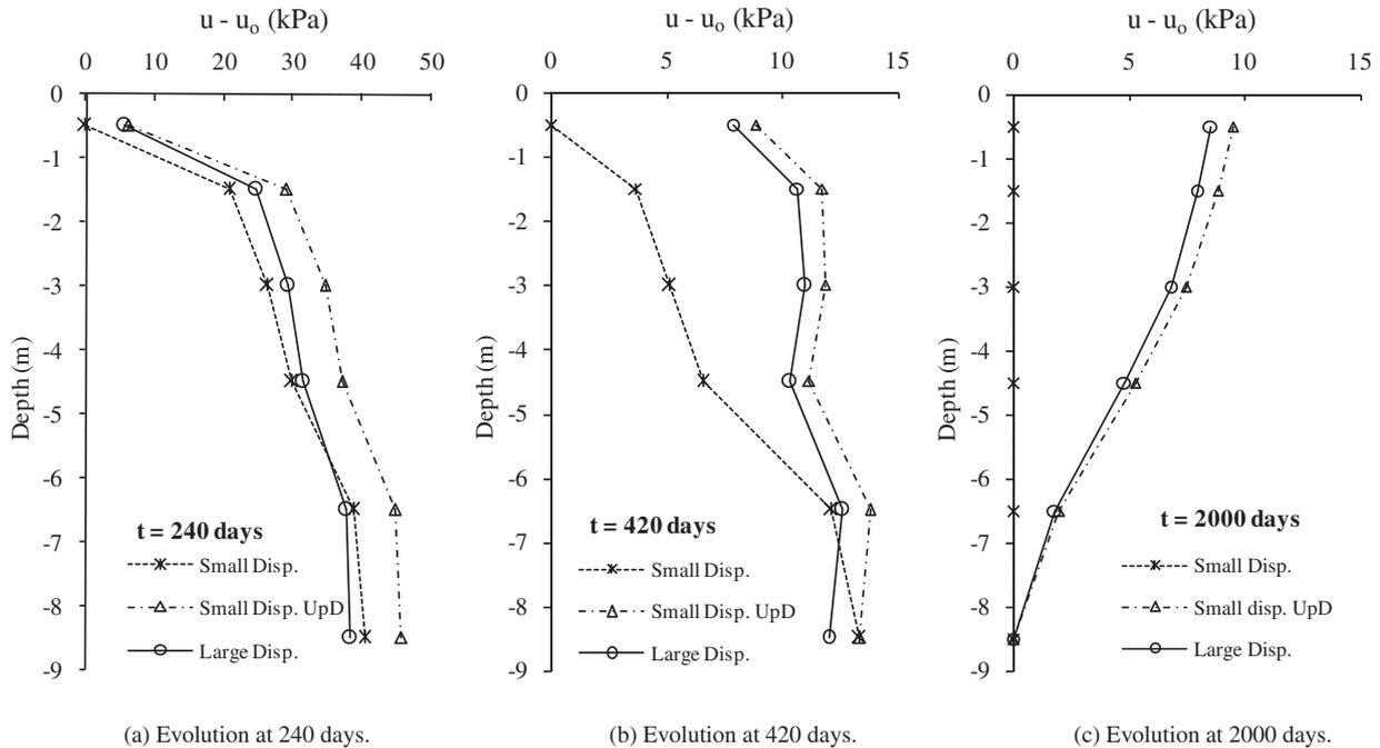
Fig. 6. Numerical predictions of  $u-u_0$  with depth.
