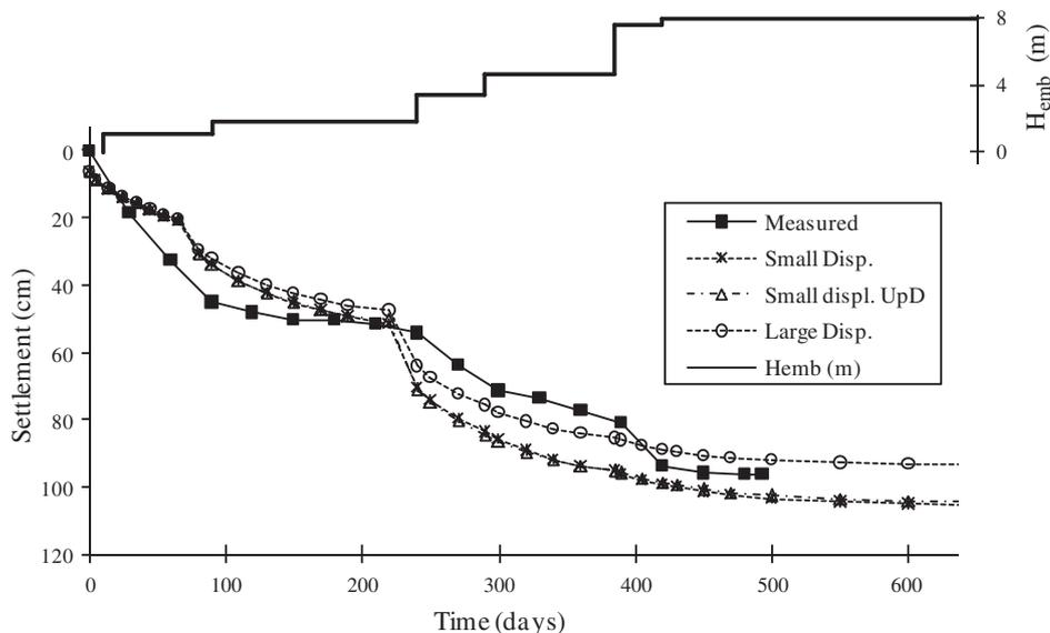
**Fig. 2.** Observed and predicted settlements (plate T).
