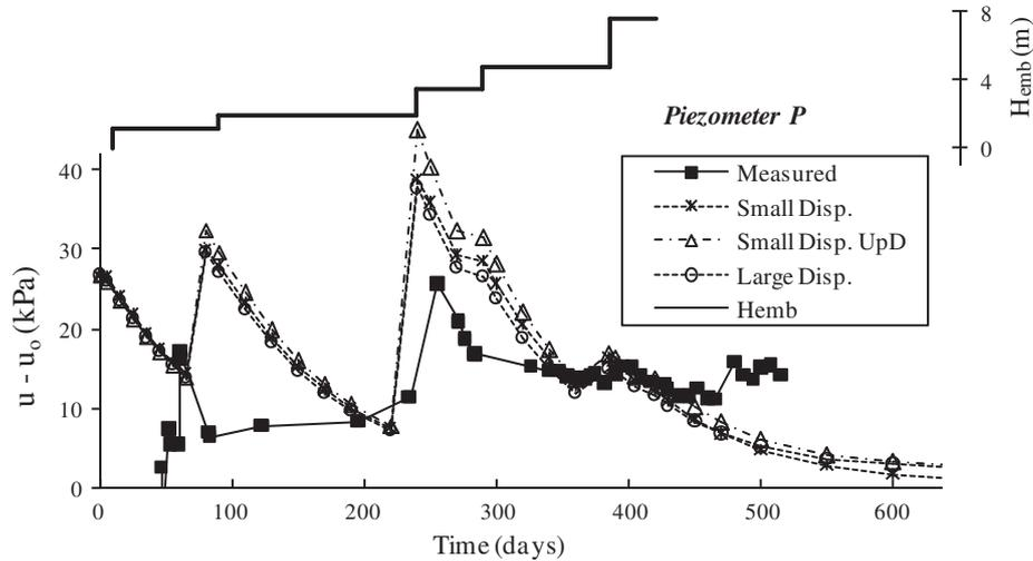
Fig. 5. Observed and predicted  $u-u_0$  in piezometer P.
