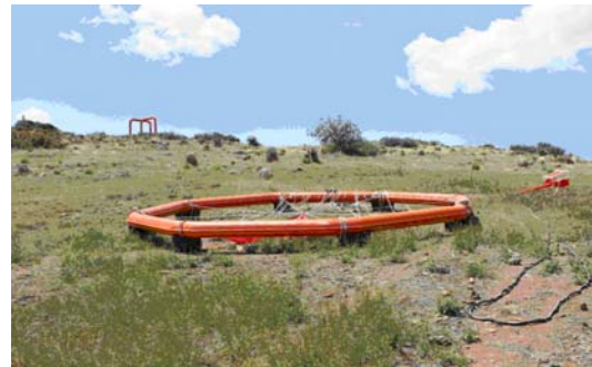
Figure 1 - picture of the airborne coil with the base station in the background.
