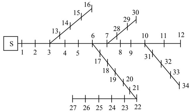
Fig. 6 34 - bus distribution network configuration
