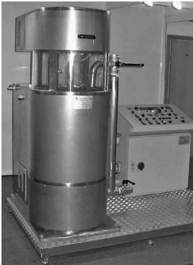
Fig. 2. The ball mill (Mill/130, Packint, Milano, Italy) used to perform experiments. Inside the double-jacket cylinder an agitator shaft moves 400 kg of wear resistant stainless steel balls, whose relative movement generates the refining action.
