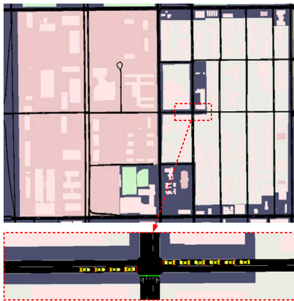
Fig. 11 Test traffic subnetwork in SUMO
