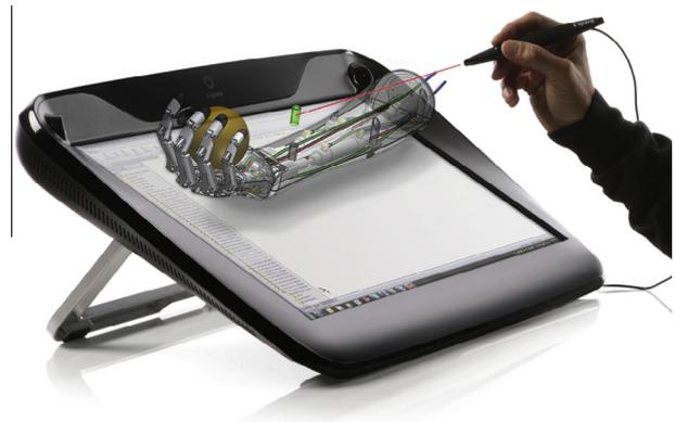
**Fig. 2.** The zSpace tablet and the custom interaction stylus [24].
