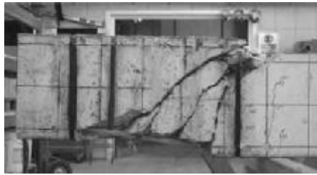
Figure 10. Shear failure of an FRP RC beam.
