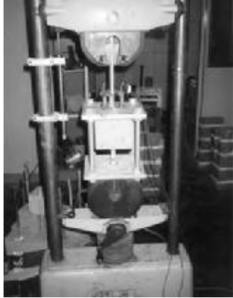
Figure 13. Pull-out test arrangement.
